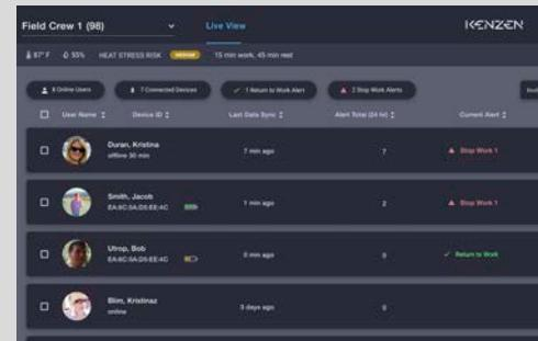
A dashboard may provide information to both the OSH professional and to the worker, often on a phone or tablet. In this case, an app provides information about heat risk to workers, including the temperature, humidity and real-feel temperature.
